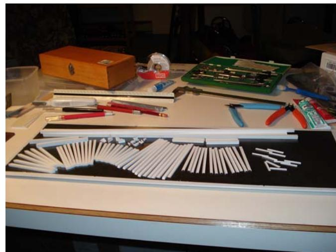
To glue everything together, I used the Tamiya Extra Thin liquid glue. This worked extremely well and provided strong joints and set up quickly. Before gluing, I made a base from a piece if 1/8" thick steel. I laid out a full size 1/25 print of the drawing on the
