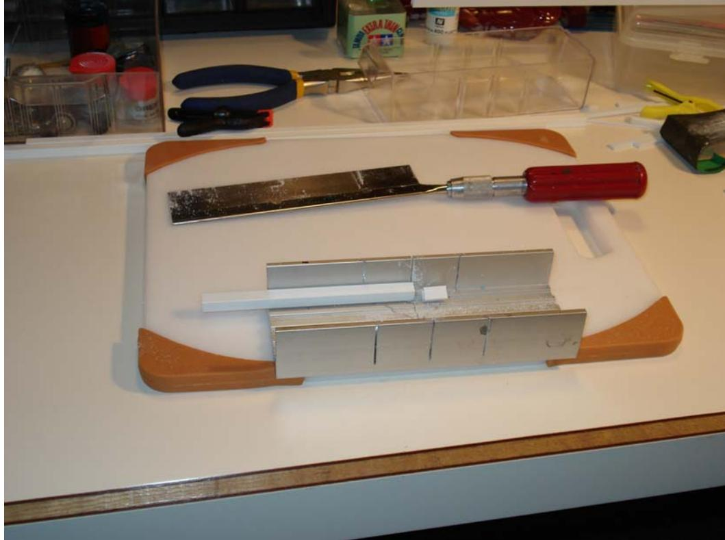
Since some of the parts had an angle of more than 45 degrees, a jig for the razor saw had to be made.
