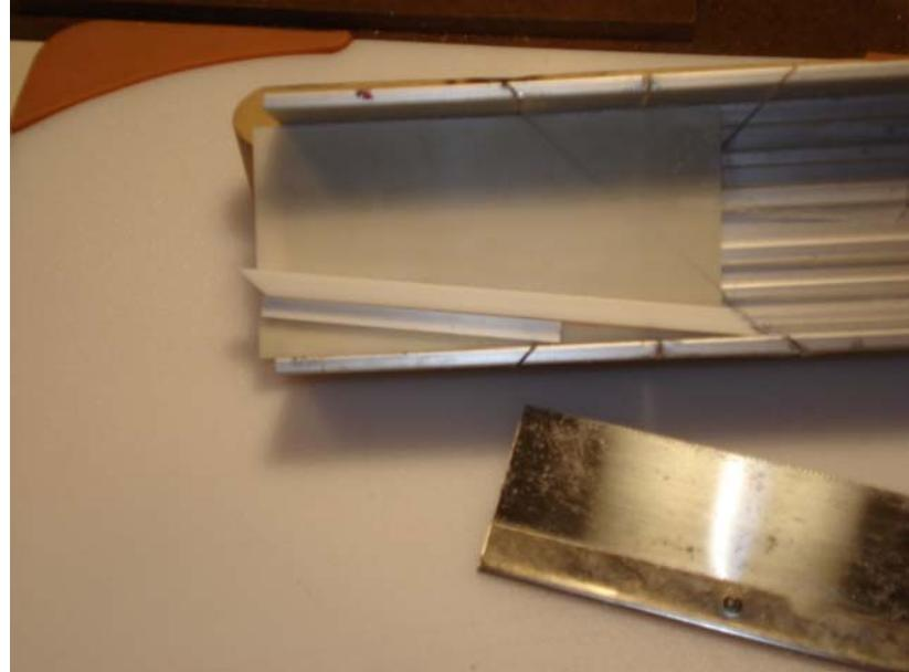
The small parts were cut using a 'Chopper' from North West Short Line. To get the ends perfectly square or angled precisely, the 'True Sander' from North West Short Line was used.
