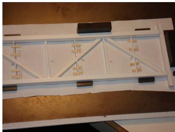
base and used magnets to align the pieces for gluing. Once the pieces were aligned, the extra thin glue was applied from the top by touching the joint with the applicator brush and capillary action pulled the glue throughout the joint. Where the cross members were in the center of the chord members, shims had to be placed under them prior to gluing.
